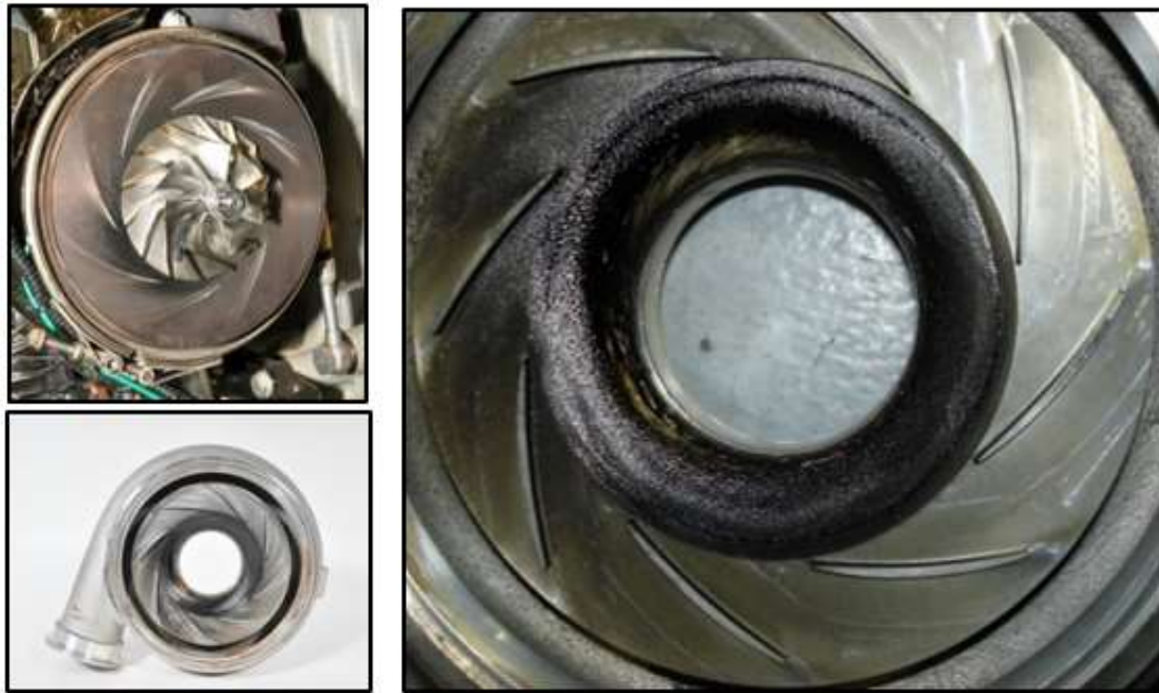
CCV Impact on compressor after 200 h durability cycle using current state of the art crankcase breather with closed crankcase system.
